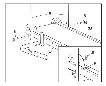
CAUTION: If the Cotter Pins (8) are not inserted into the Long Pins (5) as shown, the Long Pins may slip out, resulting in injury to the user.
